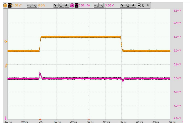
图 7.8 线性瞬态响应 (5V to 10V, V_{OUT}=5V , I_{OUT}=0mA )
