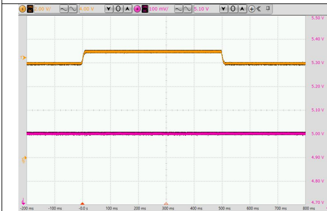
图 7.7 线性瞬态响应 (8V to 9V, V_{OUT}=5V , I_{OUT}=0mA )
