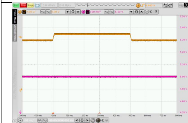
图 7.7 线性瞬态响应 (8V to 9V, V_{OUT} = 5V , I_{OUT}=0mA )
