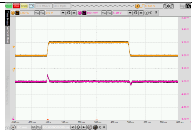
图 7.8 线性瞬态响应 (5V to 10V, V_{OUT} = 5V , I_{OUT}=0mA )
