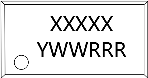
Fig.D.1 SOT23-5/6 顶部印记
