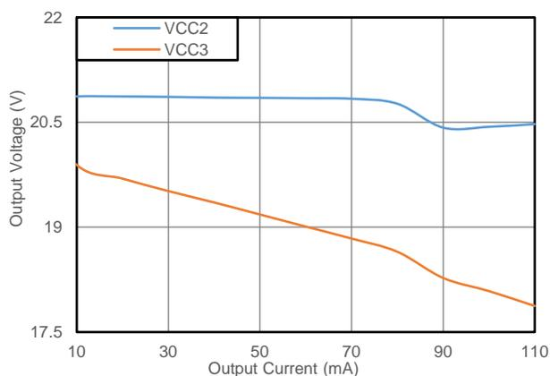
图 5.5 输出电压 vs 输出电流 (lout1 空载)
