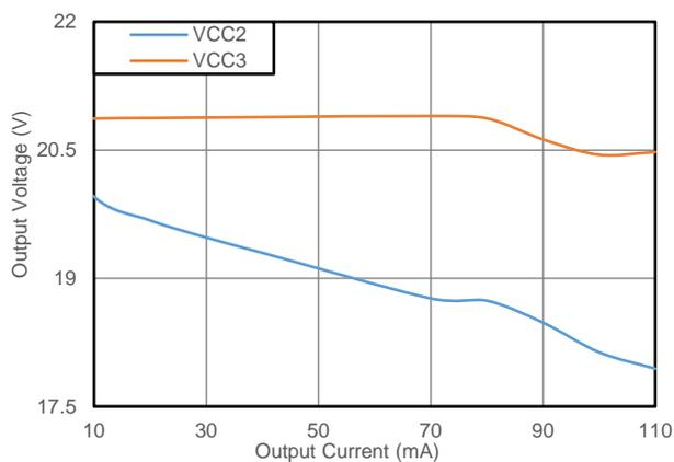
图 5.3 输出电压 vs 输出电流 (lout2 空载)
